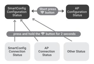
Power on the device, reset Wi-Fi, and select a connection mode.
