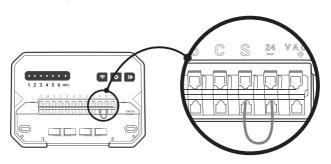
• Separately connect the line of the rain sensor to port 24 VAC- and port S.
